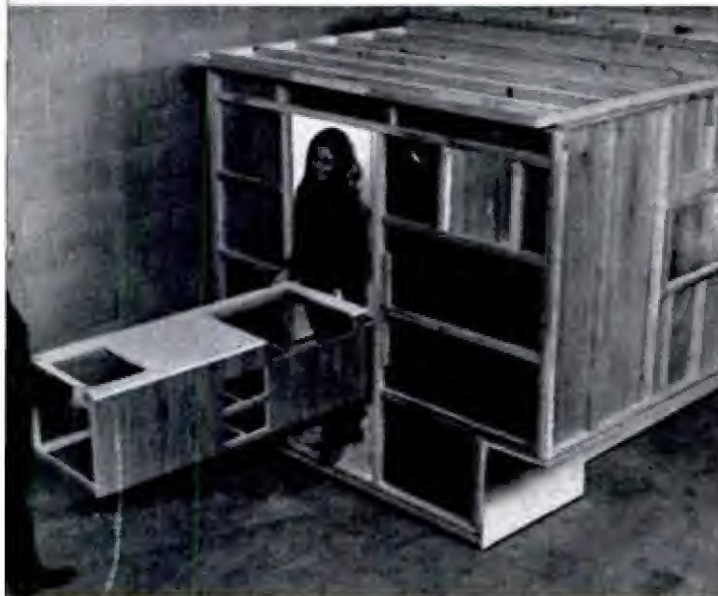
ASSEMBLED KITCHEN COUNTER is slid into place. Camper can be assembled using regular hand tools
